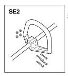
Install the handle to the shaft tube and clamp at a position best for your job. (SE2)
